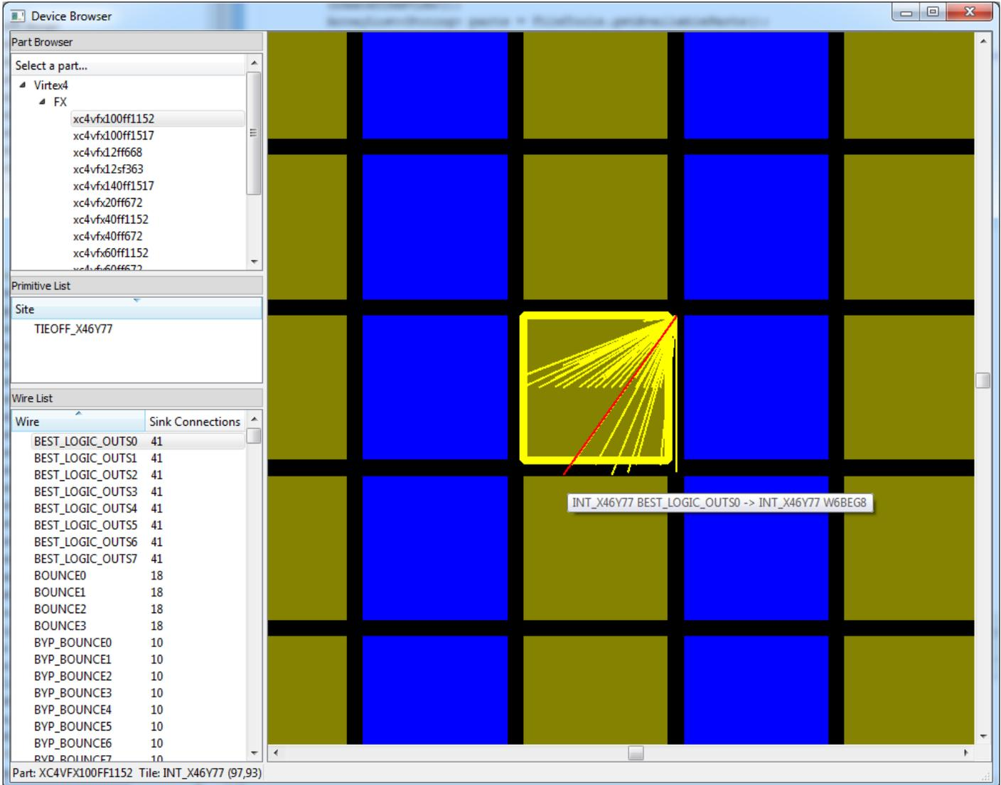
Figure 7 - Device browser screenshot showing wire connections
